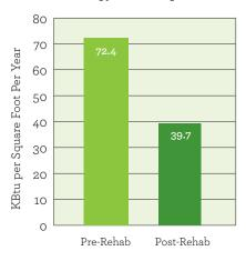
With efficient heating and cooling design and other green retrofits, the energy consumption of Viking Terrace was reduced by 45% after rehabilitation. Water usage also fell to about 43 gallons per person per day, compared to a national average usage of 69 gallons. Viking Terrace is a 60-unit building originally built in 1974.<sup>3</sup> Viking Terrace (shown on front) was renovated in 2007 by Southwest Minnesota Housing Partnership and is a Minnesota Green Communities demonstration project.
